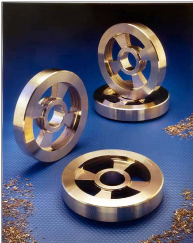
Photo 6. Continuous cast gear-wheel blanks, aluminum bronze, alloy C95400. This alloy, like other aluminum bronzes, is known for its high as-cast strength (35 ksi, 221 MPa YS; 85 ksi, 586 MPa UTS) and favorable anti-wear properties. Note that the gear-wheel spokes are cast as part of the blank, thereby reducing the extent of finish machining operations. (Photo courtesy MetalTek, Inc., www.metaltekint.com .)
