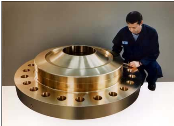
Photo 1. Centrifugally cast nickel-aluminum bronze high-pressure flange for a sub-sea weapons ejection system. Alloy C95800 was selected for this application for its combination of high yield strength (35 ksi, 241 Mpa minimum as cast), excellent seawater corrosion resistance and galvanic compatibility with mating materials. (Photo courtesy MetalTek, Inc., www.metaltelkint.com .)
